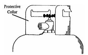
A Typical Protective Collar USING LP GASES
